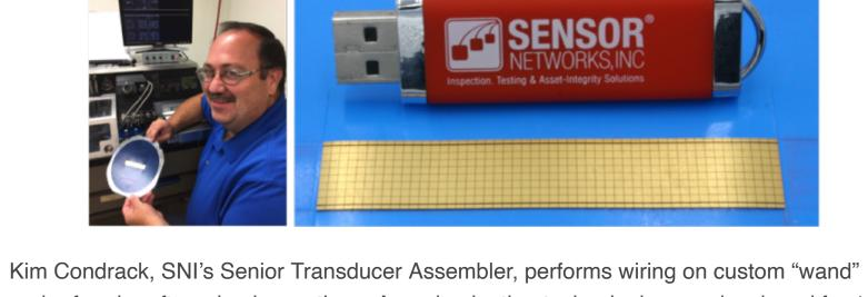
probe for aircraft-engine inspections. Array lamination technologies are developed for 16, 32, 64 and 128-element PAUT probes. This investment enhances SNI's ability to manufacture consistent, high-quality transducers in a timely fashion with improved yields. All *SensorScan* ™ transducers come packed in a rugged little box along with their certification documents.
