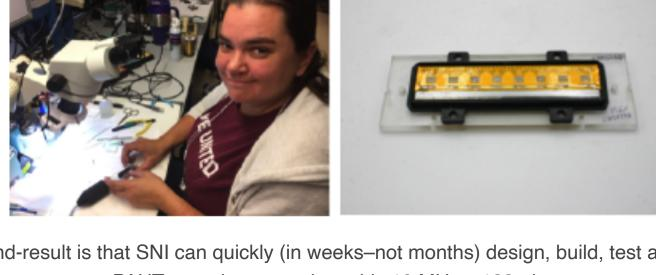
The end-result is that SNI can quickly (in weeks-not months) design, build, test and certify complex-geometry PAUT transducers such as this 10 MHz x 128-element array used for detection and sizing of High-Temperature Hydrogen Attack (HTHA) in refinery assets.
