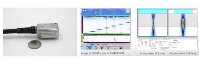
Area arrays, like the 2 x 2 x 32 element shown above can focus sound energy at varying depths and the beam can be steered in any direction to increase POD and inspection productivity. For more information or to request a demo contact Jeff Anderson, President & GM: anderson@sensornetworksinc.com. Download the *SensorScan™* Brochure below: SensorScan™ Brochure
